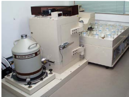
Germanium semiconductor gamma-ray detector equipped with a sample changer.
